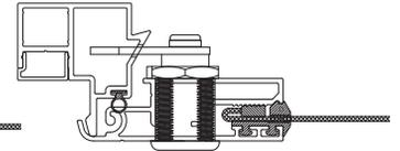
Keyed Lock Security Window Screen Cross Section
